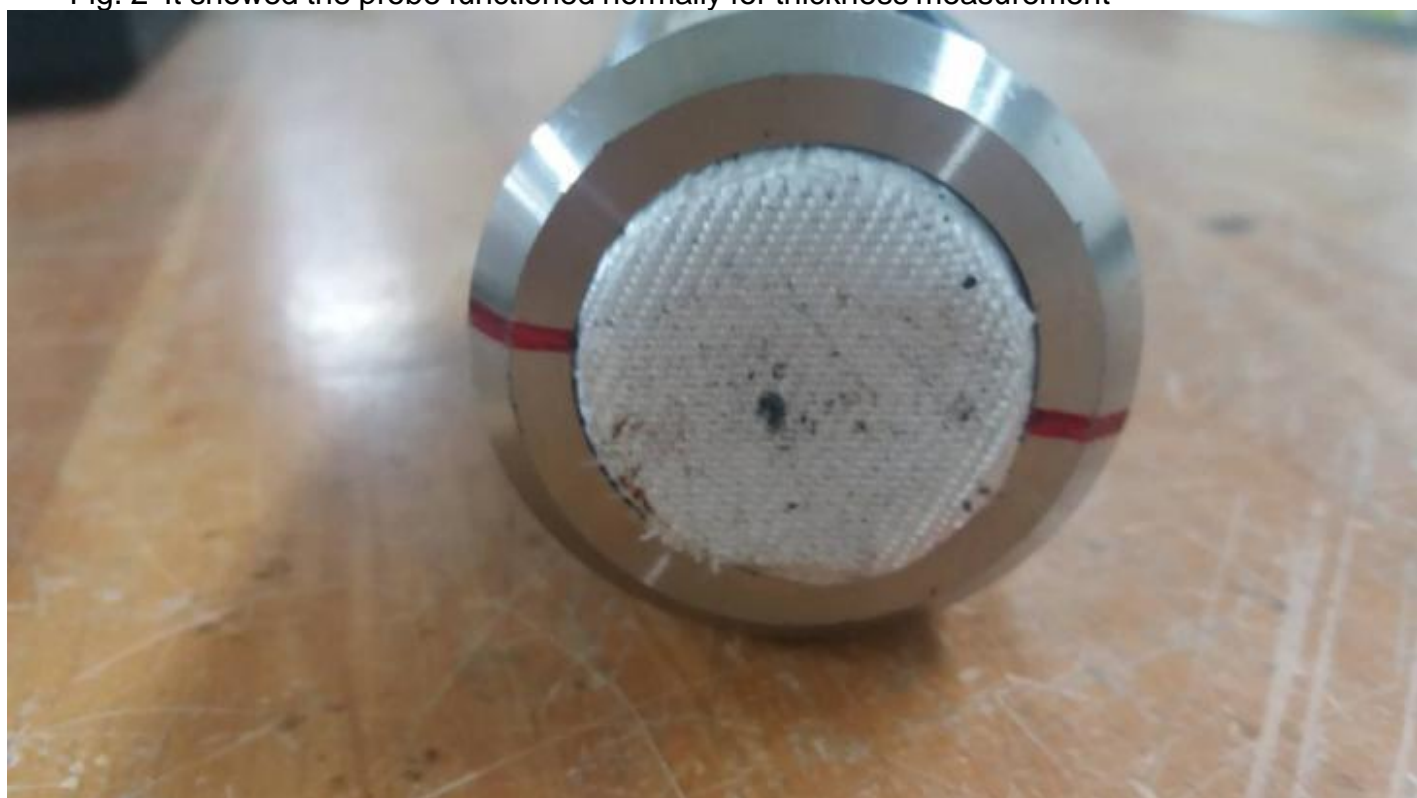
Fig.3 Figure 3 showed the probe surface outlook after tested at 200C.
