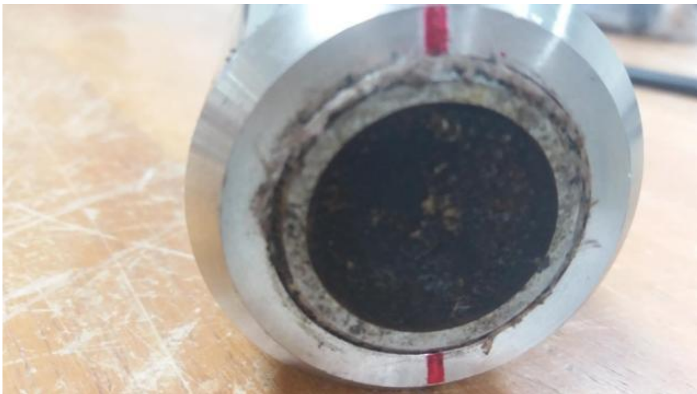
Fig. 12 Figure showed the probes surface outlook after tested at 400C (without composite protection cloth).
