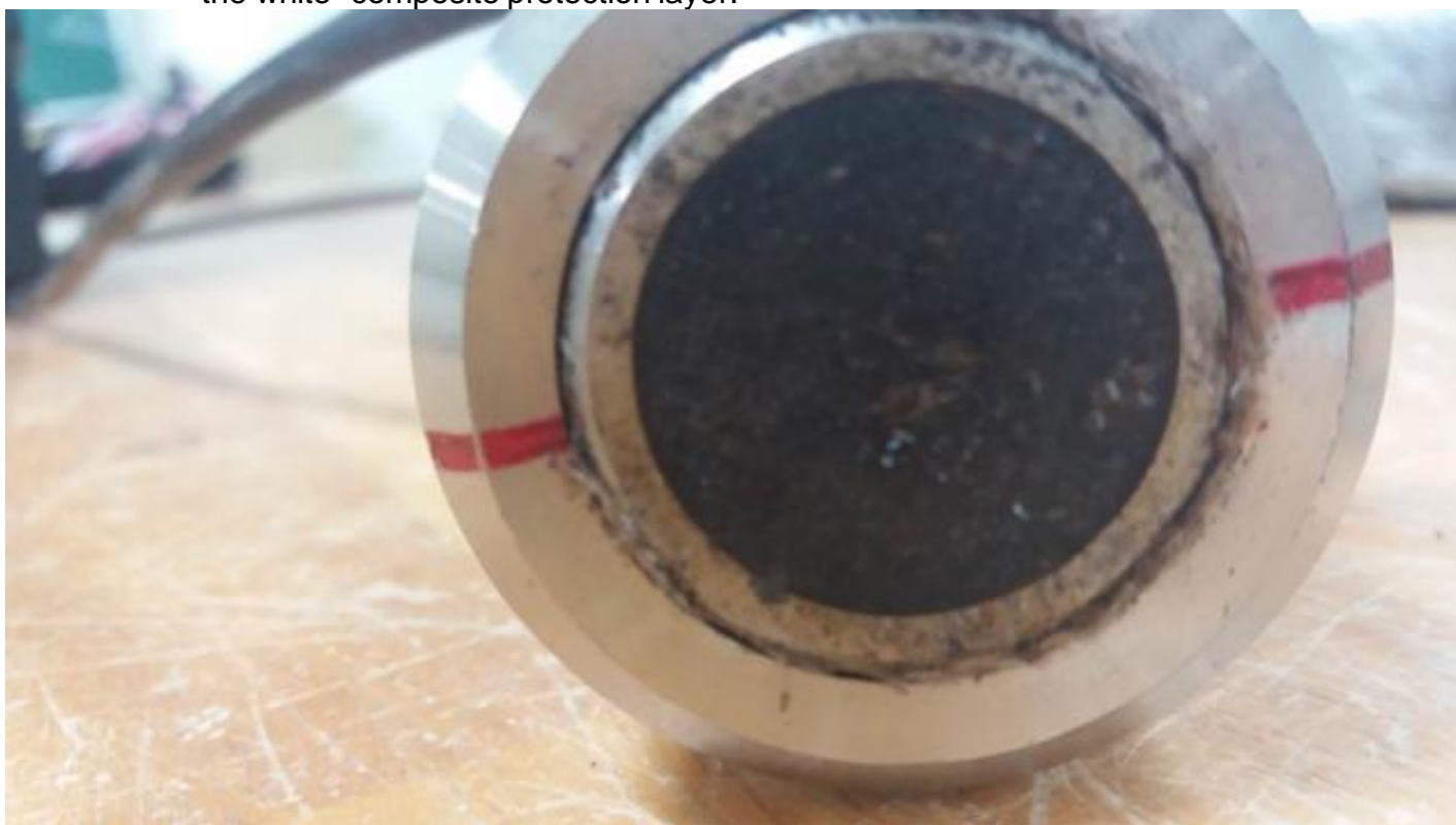
Fig. 11 Figures showed the probes surface outlook after tested at 200C (without composite protection cloth).
