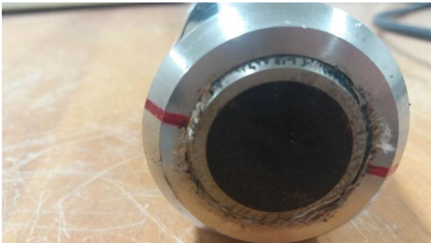
Figures 10 Figures showed the surface outlook after testing at 860C and then removing the white composite protection layer.
