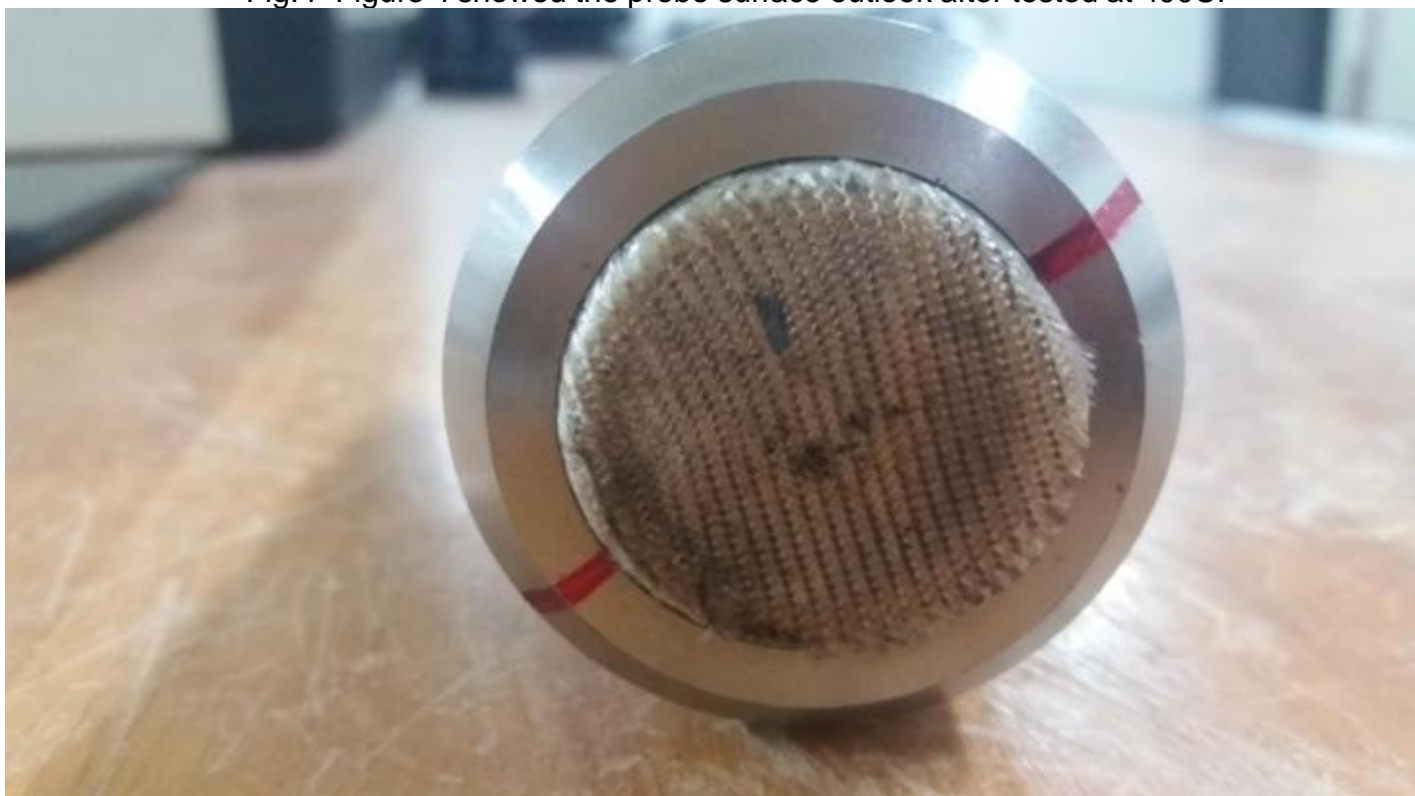
Fig.5 Figure 5 showed the probe surface outlook after tested at 600C.
