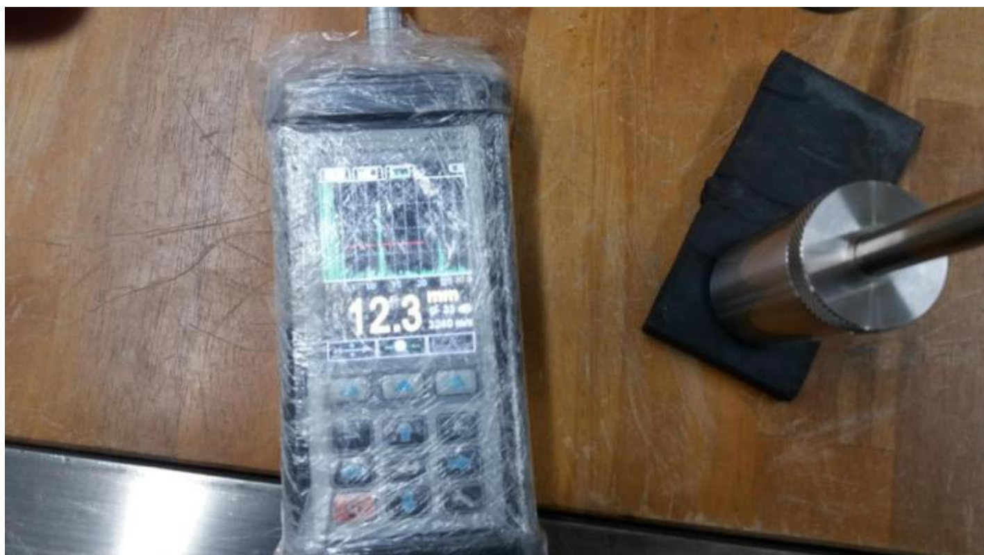
Fig. 2 It showed the probe functioned normally for thickness measurement
