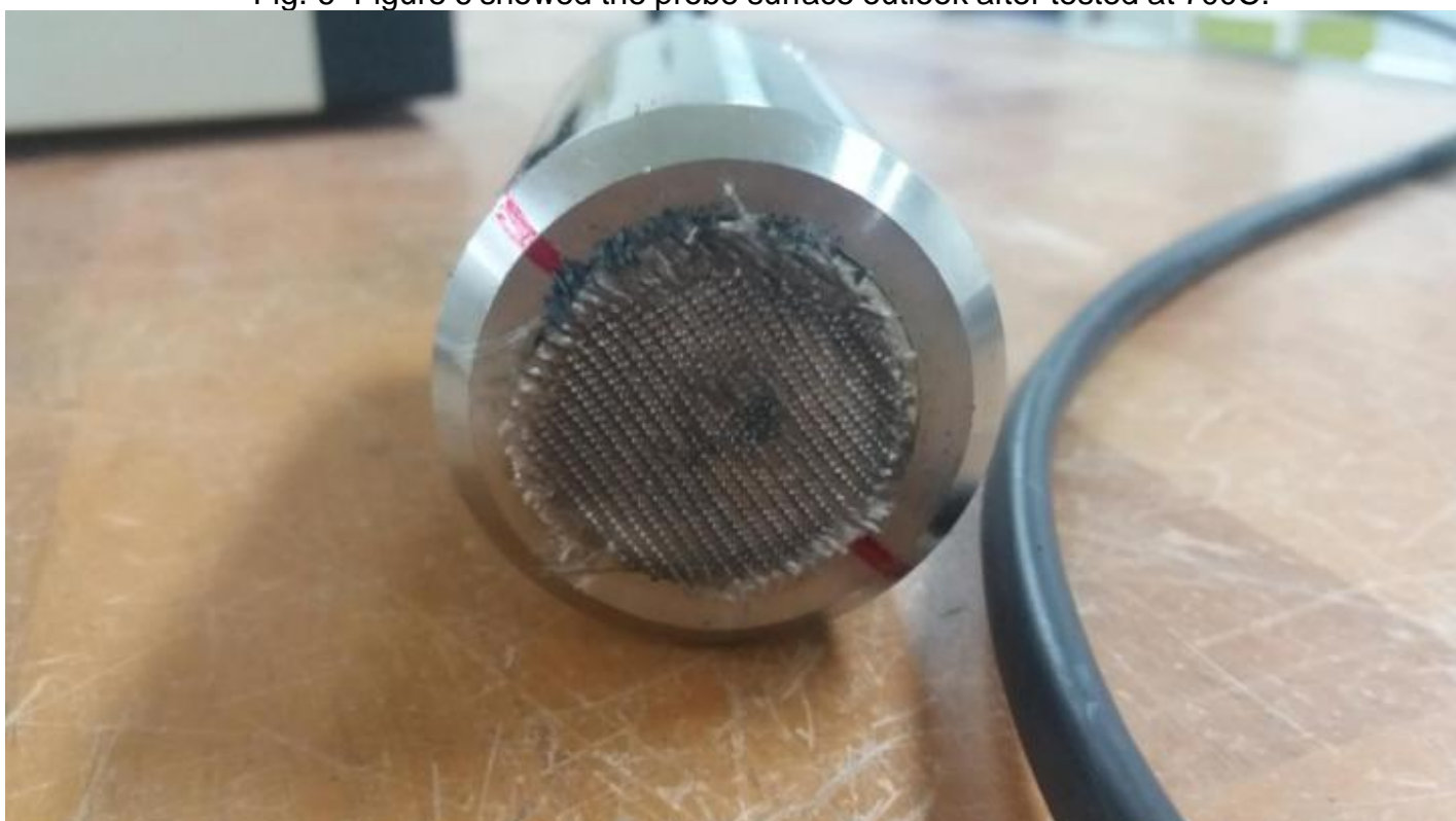
Fig. 7 Figure 7 showed the probes surface outlook after tested at 800C.
